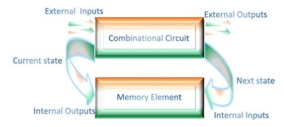
As every digital and memory circuit is built based on the finite state machines, sequential circuits are implemented for the construction of these machines. So, these circuits hold more prominence in digital and <u>electronics</u> technology.
